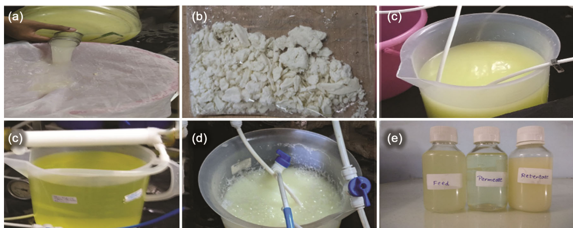
Fig. 2 — Pretreatment of raw paneer whey (a) Filtration using 200 mesh nylon filter cloth (b) Dried suspended matter of whey collected from the filter cloth (c) Permeate of filter cloth filtration (used as feed of UF process) (d) Membrane used for UF and permeate of UF (used as feed of FO process) (e) Reject or Retentate of UF of whey (f) Comparison showing difference in colour and texture of whey after UF process
