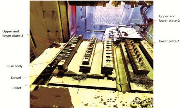
Fig. 10 — Machining of work parts using B-Type fixture
