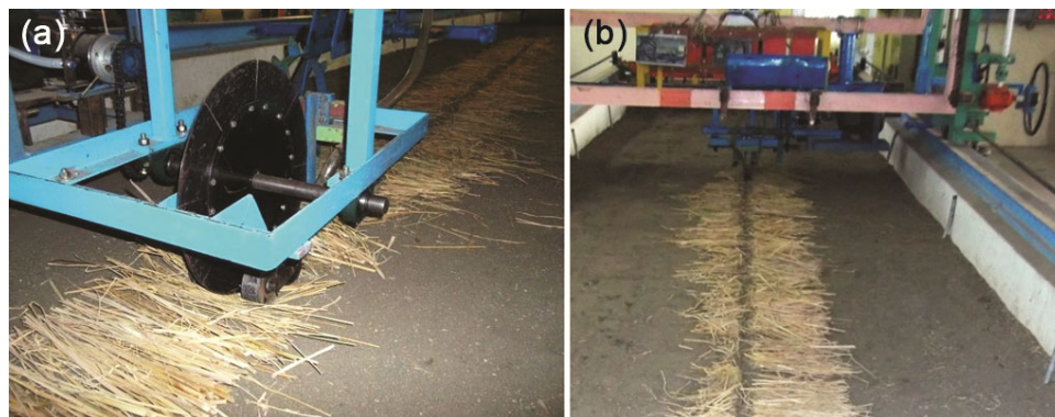
Fig. 5 — 100 % cutting achieved by plain disc coulter with pair of press wheels
