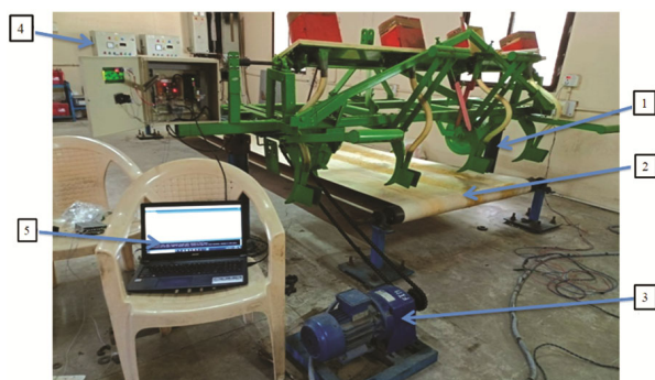
Fig. 3 — Laboratory calibration of cotton planter fitted with embedded system
