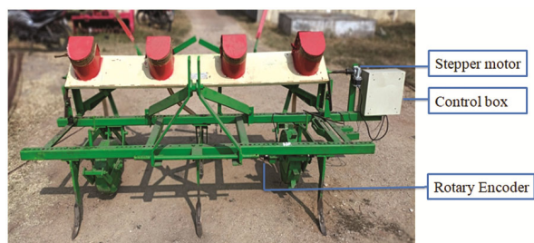
Fig. 2 — The cotton planter fitted with embedded system
