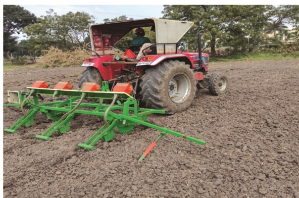
Fig. 4 — Field evaluation of cotton planter fitted with embedded system
