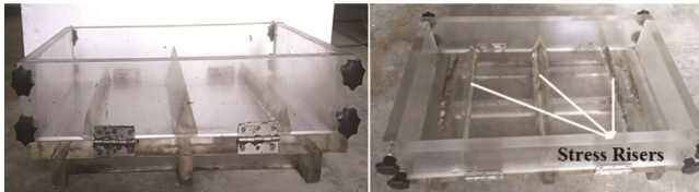
Fig. 2 — Mould for Plastic shrinkage testing
