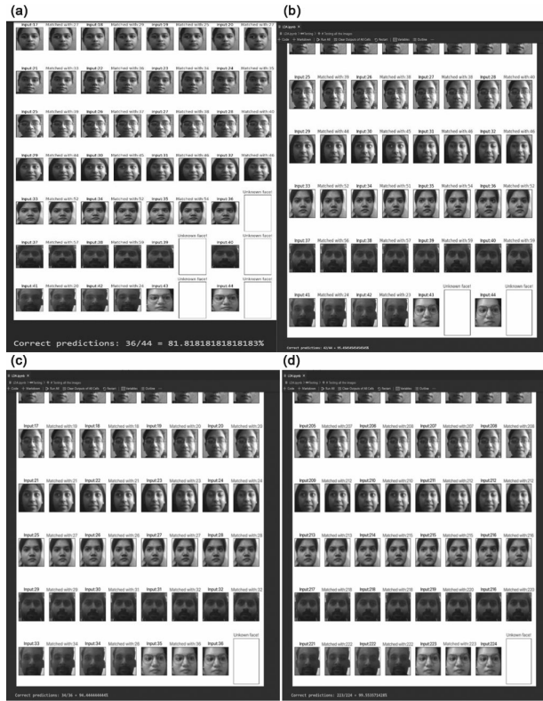
Fig. 4 — Predicted results using: (a) PCA, (b) LDA, (c) Softmax + CNN, and (d) proposed Haar Cascade + Softmax + CNN algorithms, respectively
