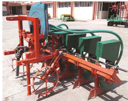
Fig. 3 — Prototype of planter for soybean planting at speed upto 1.94 \text{ m} \cdot \text{s}^{-1} ( 7 \text{ km} \cdot \text{h}^{-1} )
