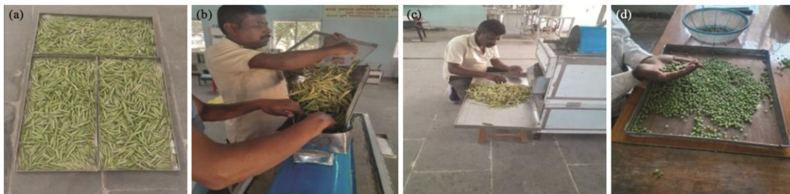
Fig. 2 — Depodding of green pea using the pea depodder: (a) Green pea pods with different moisture content, (b) Feeding through hopper, (c) deseeded pods, (d) green pea after depodding
