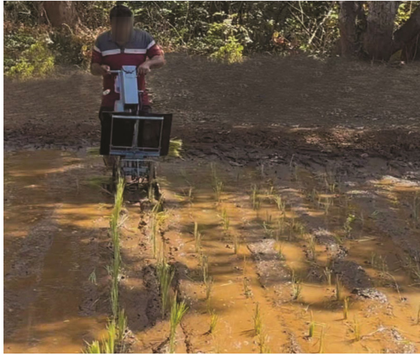
Fig. 7 — Field evaluation of developed e-powered paddy transplanter
