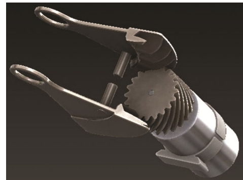
Fig. 6 — Primary motor with helical gears
