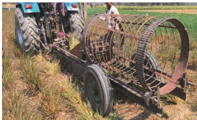
Fig. 5 — Vetiver root digging equipment in the field condition
