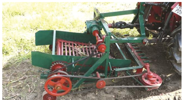
Fig. 4 — Field performance evaluation of onion de-topper cum digger
