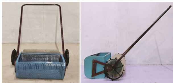
Fig. 8 — Developed prototype mechanical type neem picker collector
