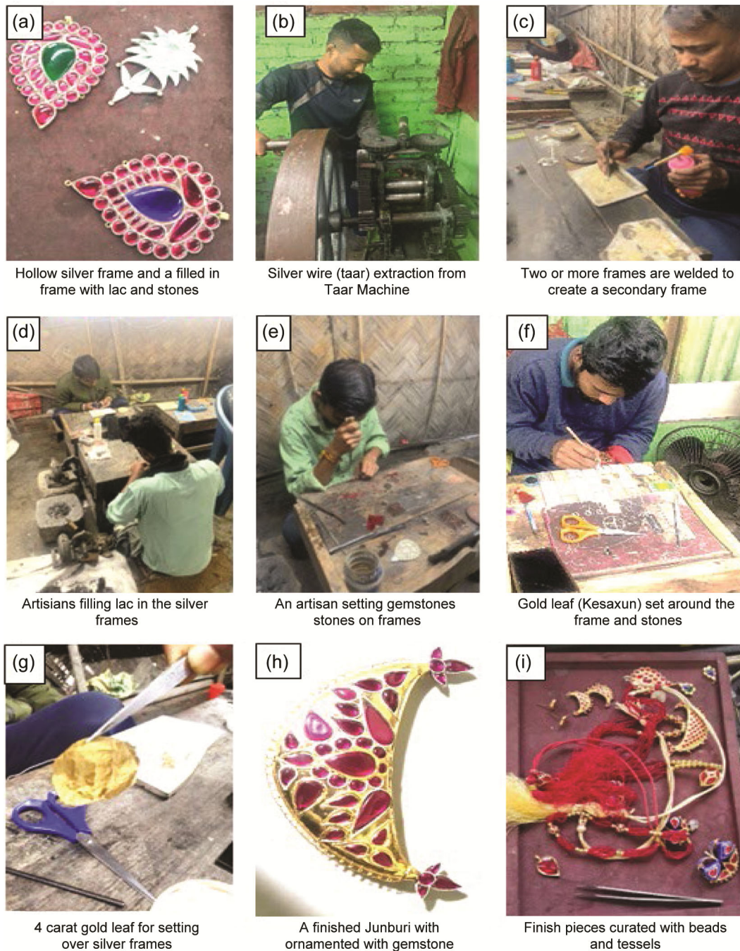
Fig. 4 — Various stages of making Traditional Assamese Jewellery
