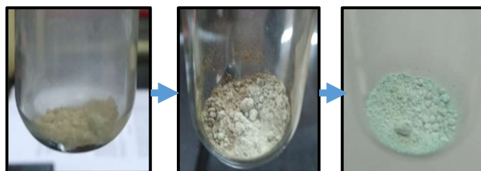
Fig. 5 Colour Change in Co- BDC MOF during CO 2 adsorption
