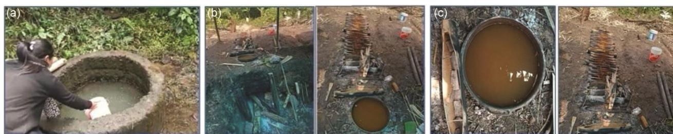
Fig. 3 — (a) Collection of brine, (b) Boiling of brine in makeshift wood-fired stoves, (c) Setting the thick brine slurry in splitbamboo tubes, The process involved in traditional salt-making
