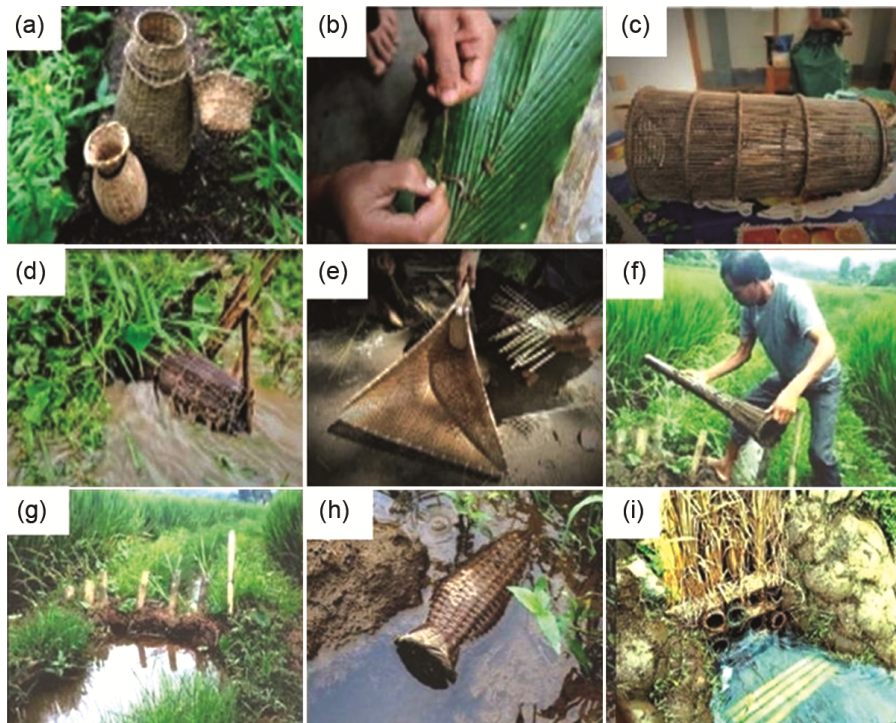
Fig. 3 — Different types of traditional fishing gears such as (a) Lanap with different designs, (b) Khwai-kynjrom , (c-d) Khoh-nam placed against water current, (e) Jakhoi , (f) laying of Khoh kha , (g) Paron , (h) Kroh , and (i) Fog 15 Kroh
