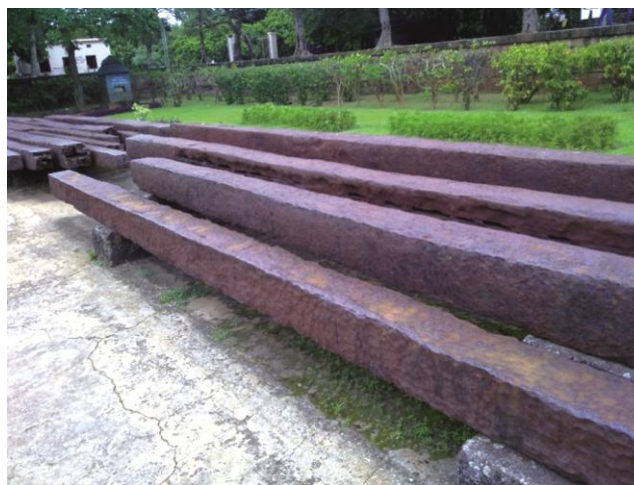
Fig. 5 — Iron beams placed in Konark's Sun Temple at Konark. Reproduced under a Creative Commons Attribution-Share Alike 4.0 International license
