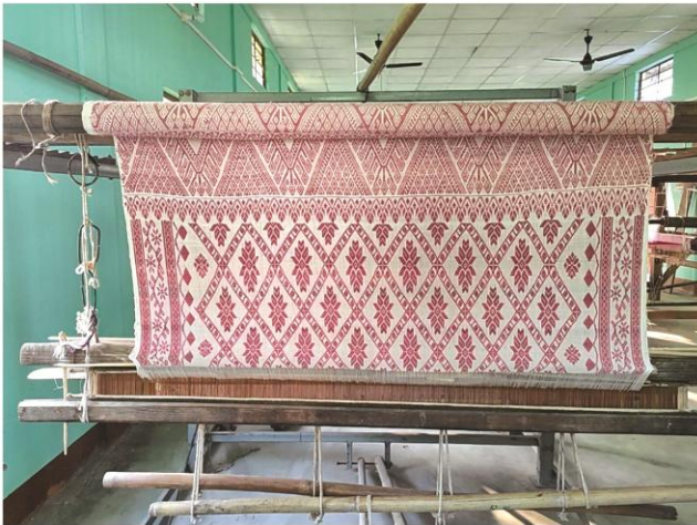
Fig. 6 — Goxain Kapur yarn specification: 2/20s organic cotton for warp & weft and 2/20s vegetable dyed organic cotton for motifs. Yarn provided by Orient Processors Private Limited, Lohra, Guwahati. Textile woven by UGC STRIDE Master Weaver Ms. Runa Bora Baruah of Jamugurihat under the guidance of Shri Bhaba Goswami, Satradhikar of Sessa Satra in Sootea, Biswanath district, Assam. Weave pattern: Plain weave
