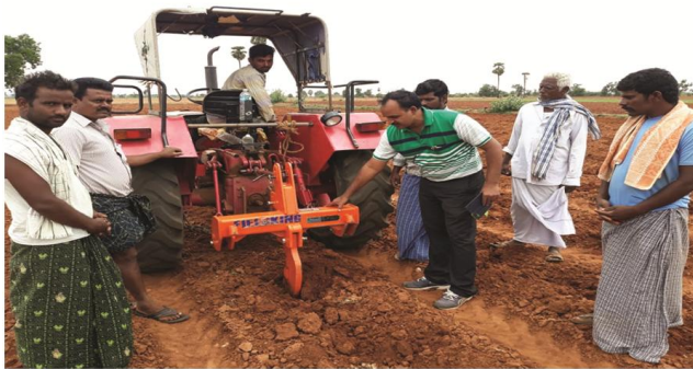
Fig. 2 — Sub soiling with chisel plough
