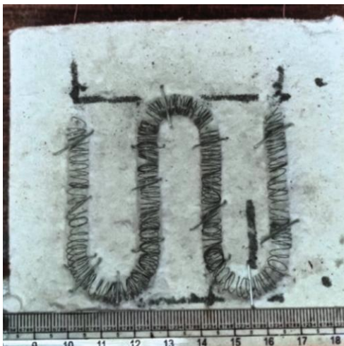
Figure 3 — The heater prepared using the nichrome wire (0.1 mm) spread in an area of 6.5 x 6.5 cm
