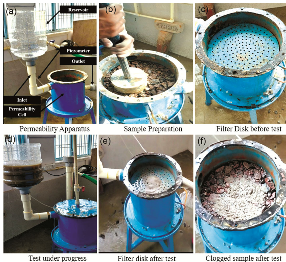
Fig. 4 — Laboratory test for permeability measurement under cyclic clogging with road dust.
