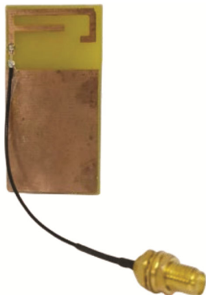
Fig. 5 — Final fabricated prototype of the proposed antenna along with SMA cable and connector
