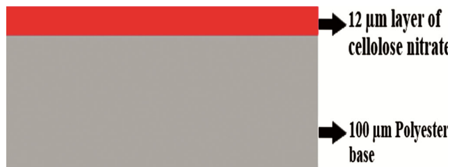
Fig. 1 — Basic schematics of LR-115 SSNTD.
