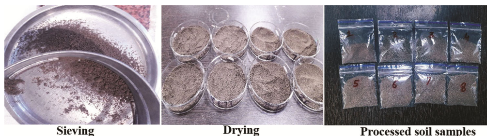
Fig. 2 — Pre-processing of soil samples.
