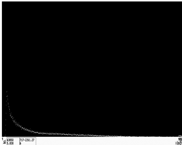
Fig. 2 — Analysis of Gamma spectrum of 10% fly ash with 90% Clay specimen.
