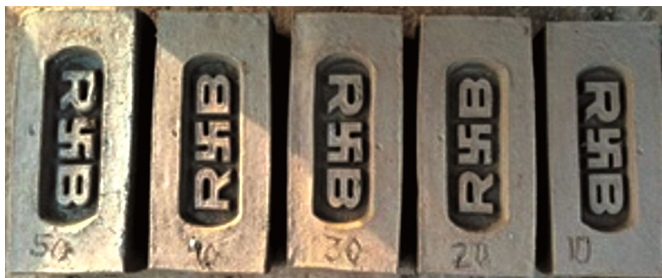
Fig. 1 — Different compositions of clay fly ash bricks.
