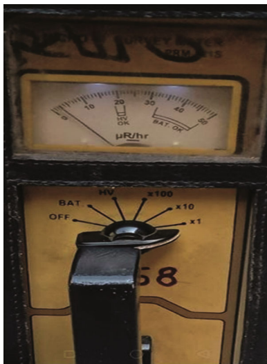
Fig. 5 — GSM used to detect Gamma dose
