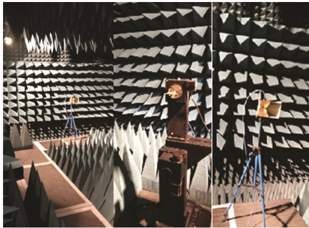
Fig. 19 — Experimental setup of transmitting and receiving designed antenna in anechoic chamber
