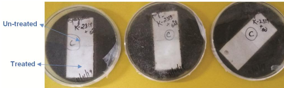
Fig. 4 — Experimental set up for determination of anti-fungal potency on white cement panel.
