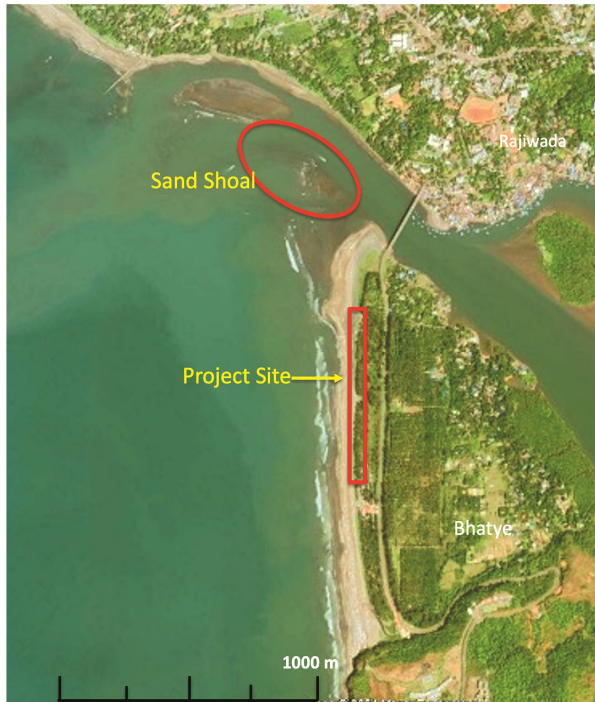
Fig. 6 — Sand shoal dredged for dune nourishment at Kajali river inlet adjoining Bhatye beach
