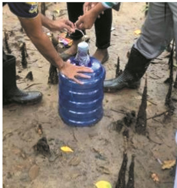
Fig. 2 — Gas trapped using a chamber
