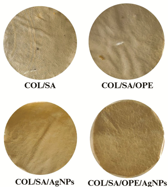
Fig. 1 — Visual images of COL/SA-based biocomposite film
