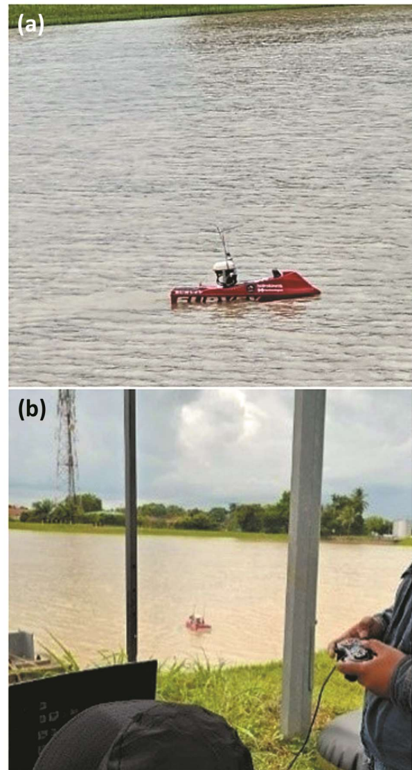
Fig. 5 — Autonomous hydrographic survey operation: (a) USV Suraya 1 (Class USV 1.08 m); and (b) Shore-based ground station for control and data acquisition
