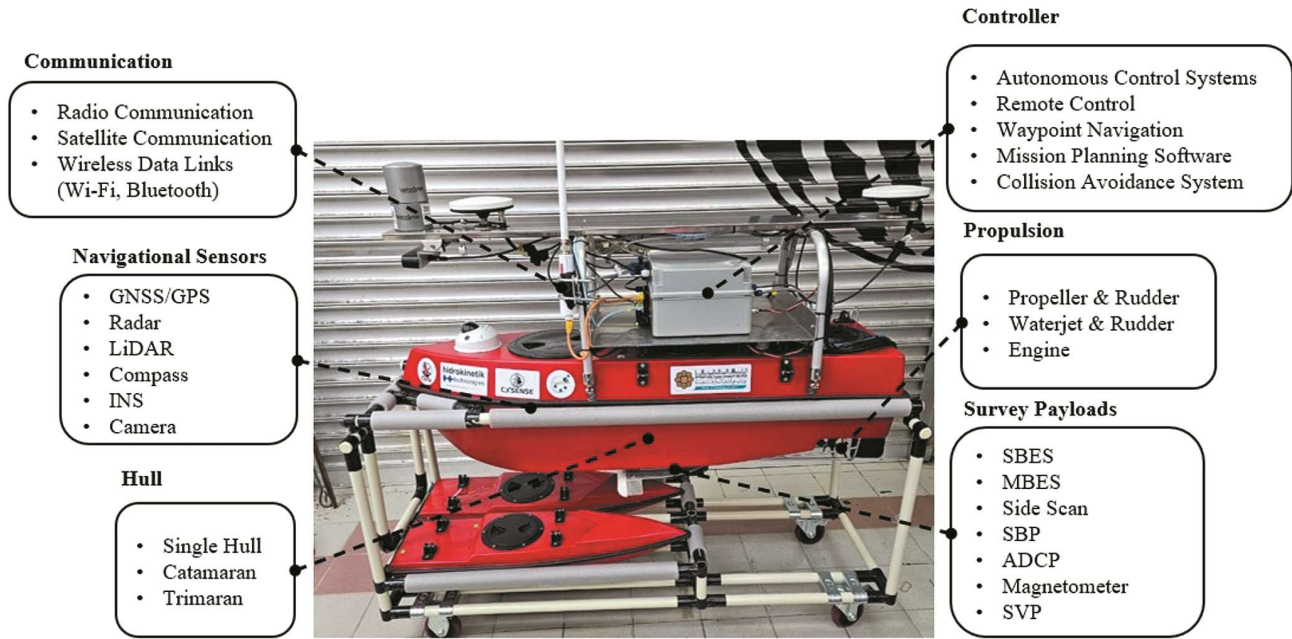
Fig. 6 — Conventional hydrographic USV configuration: Illustrates the typical setup including communication antennas, navigational sensors, hull design, control systems, propulsion units, and survey payloads
