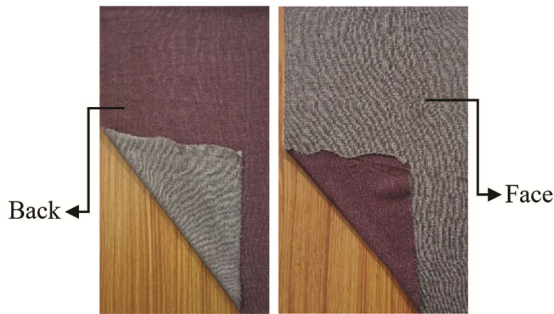
Fig. 1 — Single jersey knitted structure
