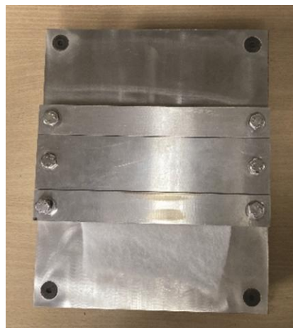
Fig. 1 — Lindsley's instrument to measure fibre orientation
