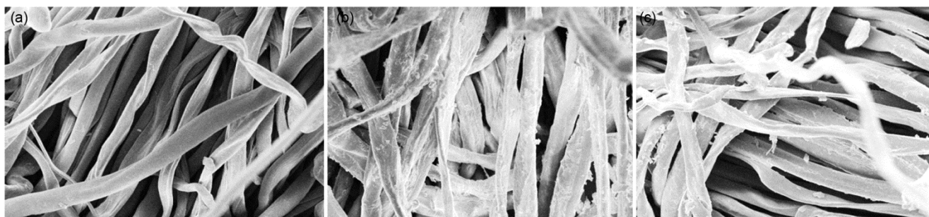
Fig. 7 — SEM images (500 \times ) of (a) untreated, (b) C6 based and (c) C8 based samples
