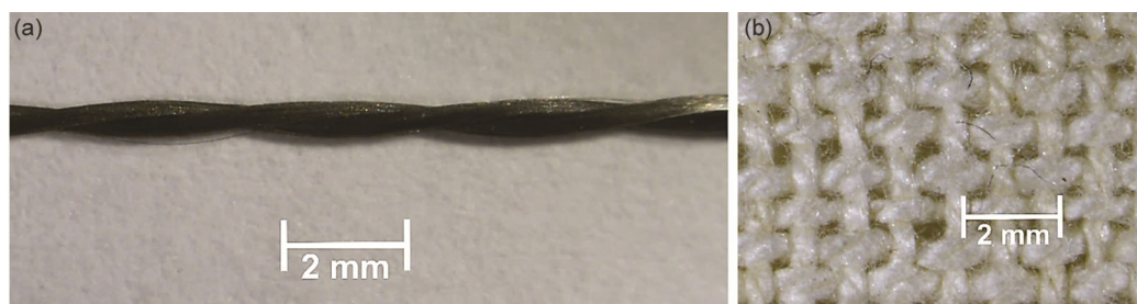
Fig. 1 — Textile material (a) 2-ply stainless steel thread and (b) plain weave woven fabric
