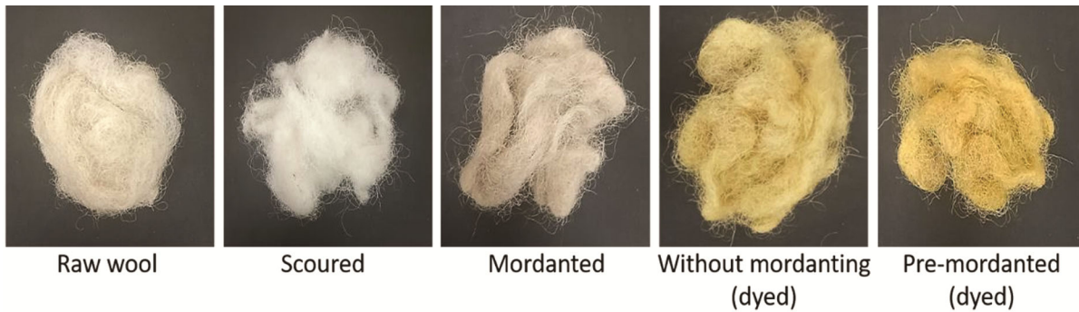
Fig. 5 — Images of raw, scoured, mordanted and Butea Monosperma dyed pashmina wool
