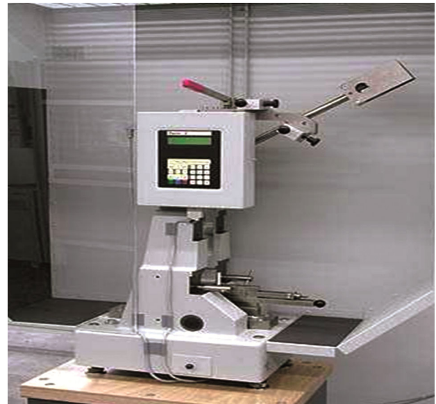
Fig. 6 — Izod Impact Test Configuration (ASTM D256)
