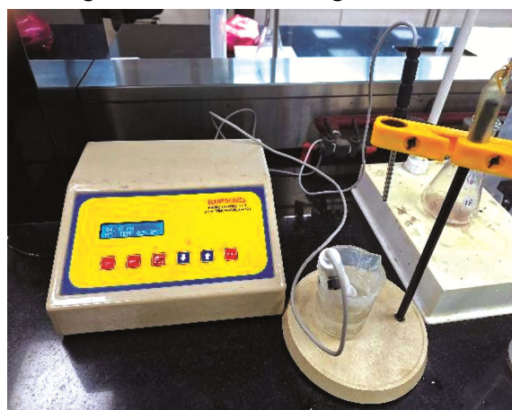
Fig. 1 — pH Meter Used for Adjusting the pH of Silane Solution
