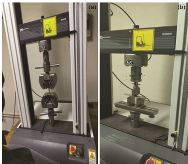
Fig. 3 — Instron 3369 UTM machine and samples set for testing (a) Tensile Test, and (b) Flexural test
