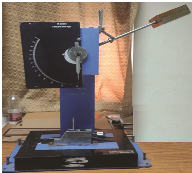
Fig. 4 — Izod impact tester with the sample set for
