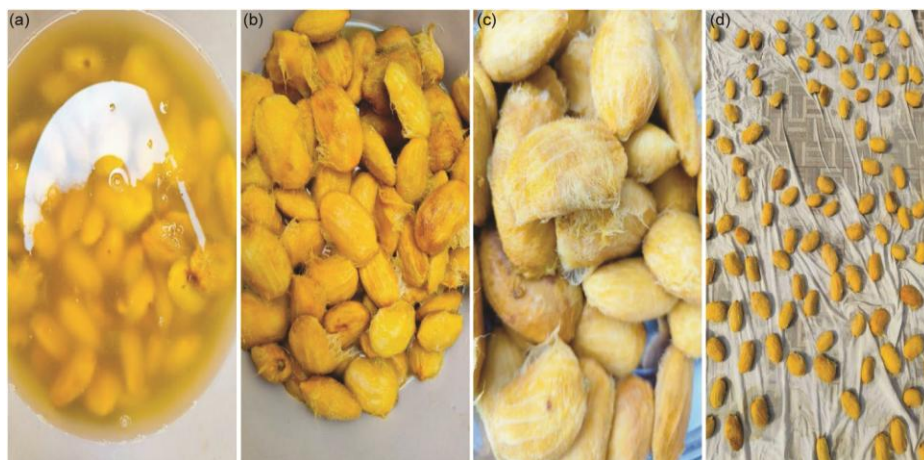
Fig. 1 — The collection and extraction of fibres from Mangifera indica seeds (a) using the water boiling and stripping method (b, c) followed by sun dry (d)
