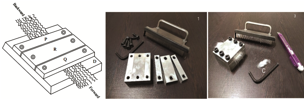
Fig. 1 — Schematic diagram of the apparatus used to determine fibre orientation
