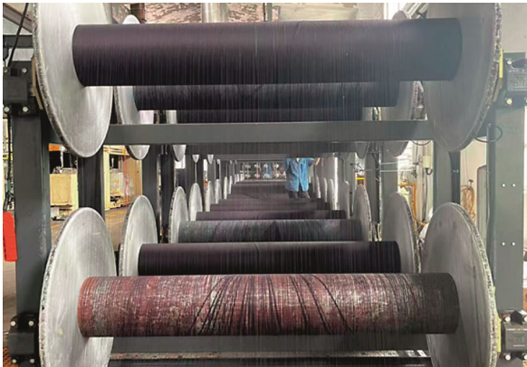
Fig. 1 — The amount of residual yarn after the unwinding in the denim product production workshop
