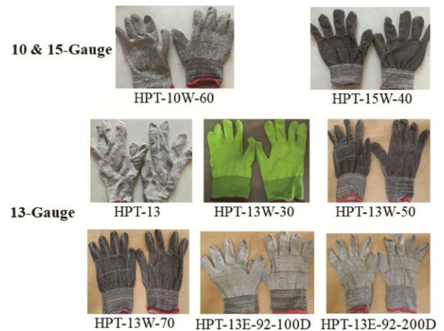
Fig. 1 — Developed glove samples on 10, 13, and 15-gauge glove knitting machine
