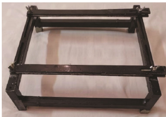
Fig. 2 — Special frame developed for applying extension
