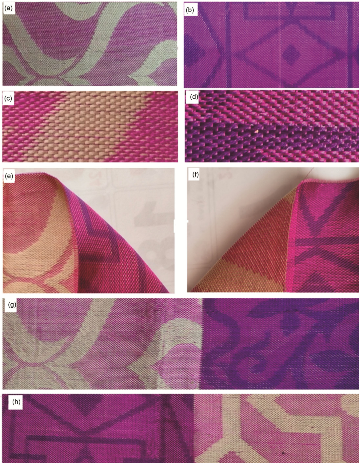
Fig. 7— Structures and appearance of DFF shawl fabric (a) ogee motif on top side, (b) diamond motif on the reverse, (c) ogee motif formed using brown and red colour picks, (d) diamond motif formed using purple and blue colour picks, (e) ogee motif on one side with the diamond motif on the reverse, (f) diamond motif on one side with the ogee motif on the reverse, (g) on the top side, interchange of brown-red picks of the ogee body with purple-blue picks of the border, and (h) on the bottom side, interchange of purple-blue body picks with brown-red border picks
