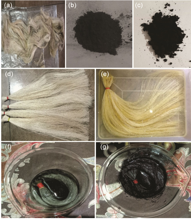
Fig. 1 — Morphological images showing (a) Untreated sisal fibres, (b) graphene oxide, (c) reduce graphene oxide, (d) sisal fibres after combing, (e) sisal fibres immersed in NaOH solution, (f) GO-coated sisal fibres and (g) rGO-coated sisal fibres
