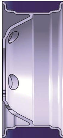
Fig. 1 — Rim (5.50 F) cross section.
