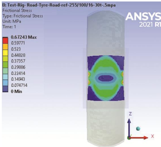
Fig. 8 — Contact pressure between rubber tire and road in test rig.
