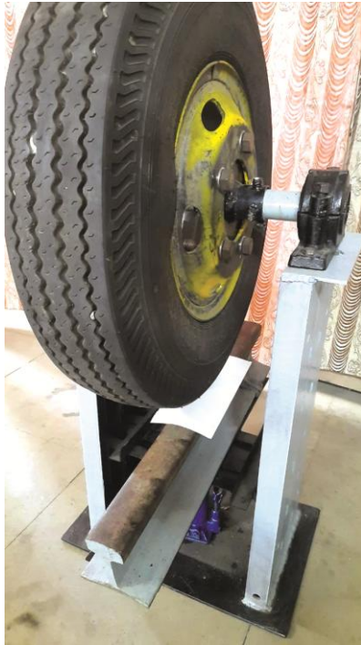
Fig. 13 — Experimentation for new rubber tire with rail using pressure paper for determining stress distribution.
