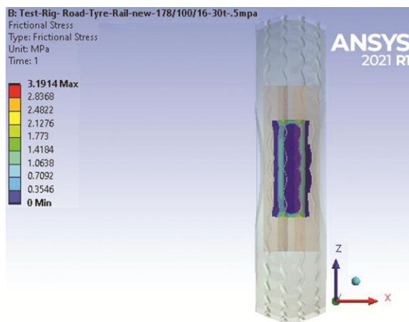
Fig. 11 — Contact pressure of rail-new rubber tire with test rig.
