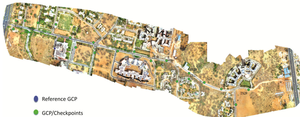
Fig. 3 — Distribution of reference GCP, ground control points (GCP) and checkpoints along the study area.
