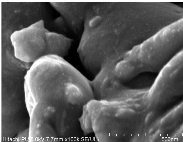
Fig. 4 — SEM image of chalcogenide Se_{78}Te_{20}Sb_2 glass.
